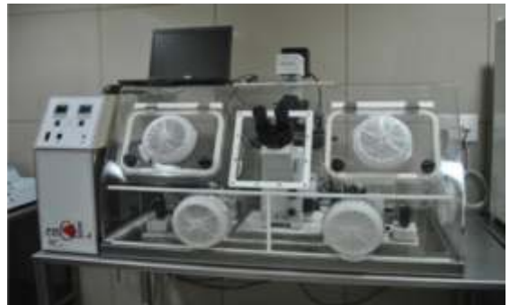
Closed Working Chamber used for ICSI. Inverted microscope in closed working chamber.
